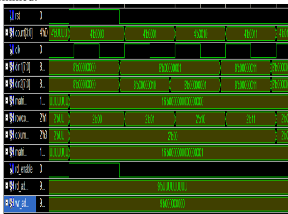
Fig.2. Timing simulation for matrix multiplication unit
