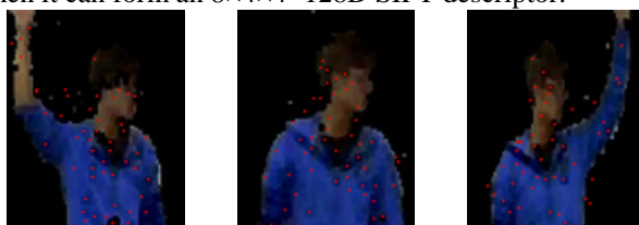
Right Hand Normal Gesture Left Hand Fig.5. Sampling of feature points by SIFT descriptors for raising hands.
