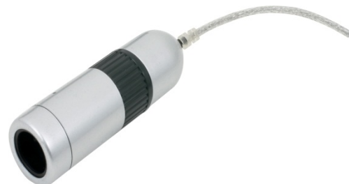
Fig.3. Digital microscope used to monitor crack during fatigue tests
