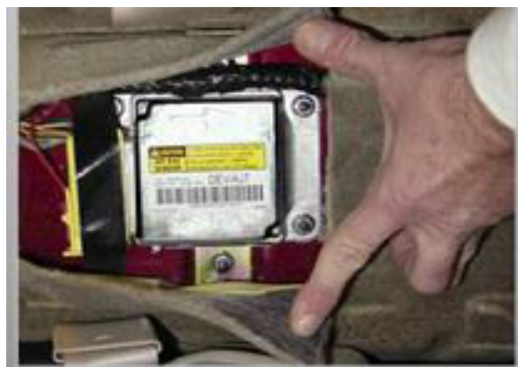
Figure 2: EDR installation under the seat
