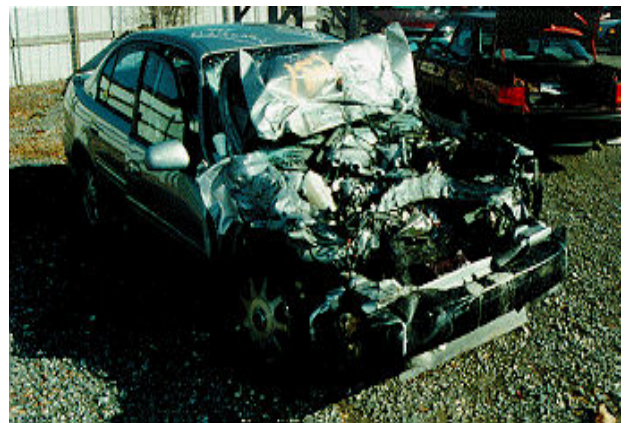
Figure 5: crash occurred in a roundabout with long collision pulse time.
