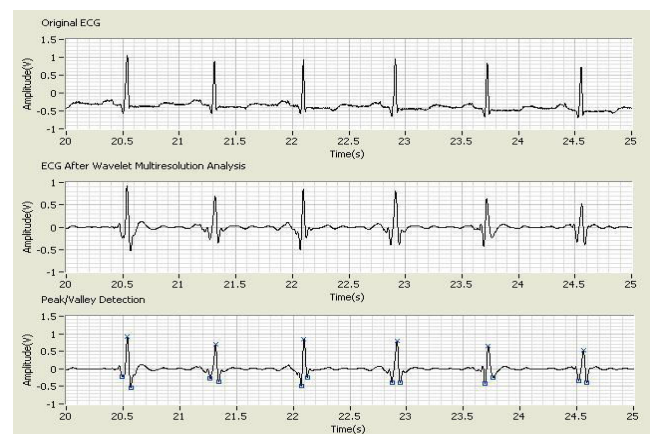
Fig iii-ECG signal after the QRS peak detection.
