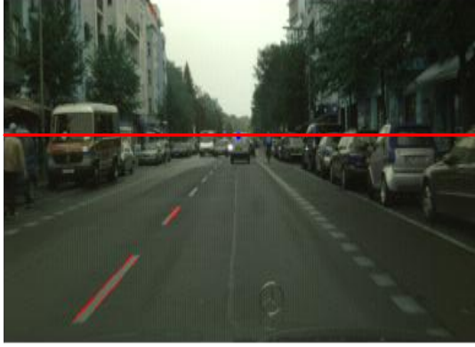
Fig. 4. Linear detection and vanishing point fitting.
