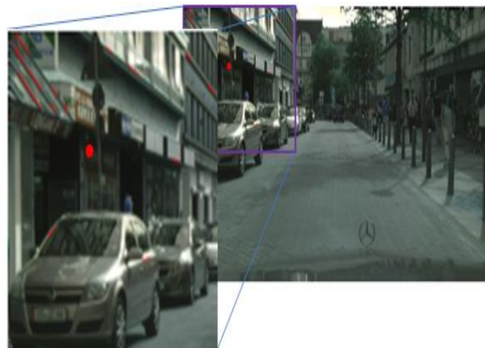
Fig. 6. Vanishing point drift caused by environmental disturbance.
