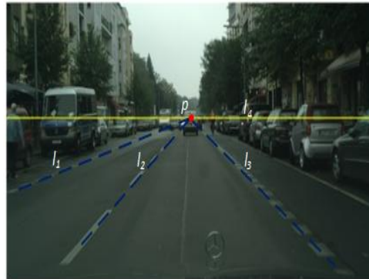
Fig. 3. Schematic diagram of linear relation and vanishing point.
