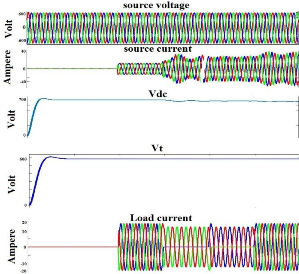
Fig. 10. Output waveforms for unbalanced linear load.
