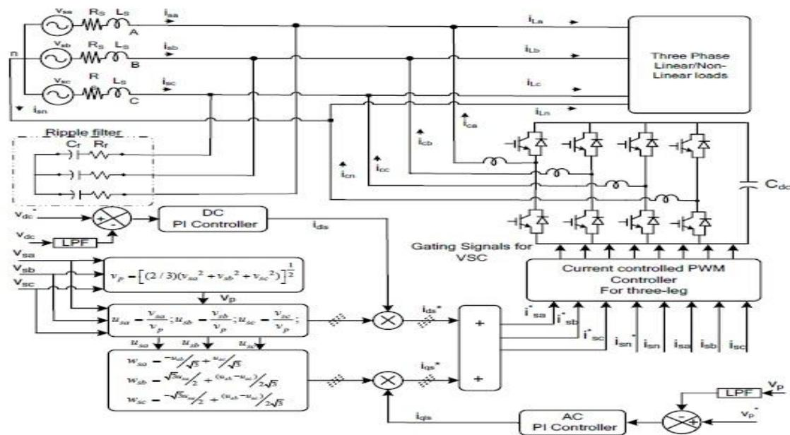
Fig. 2. Diagram of Vsc based Dstatcom with Hysteresis current control technique.
