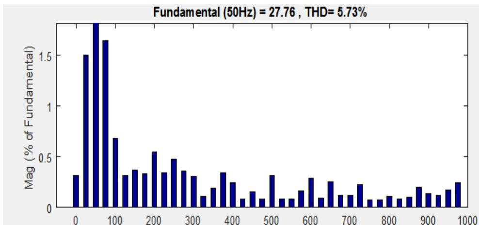
Fig. 11. Frequency analysis of compensated source current for unbalanced load shown 5.73% THD.
