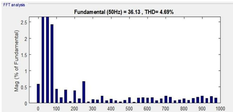
Fig. 5. Frequency analysis of source current waveform for balanced load shown 4.69% THD.
