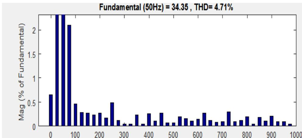
Fig. 9. Frequency analysis of source current waveform for balanced load shown 4.71% THD.
