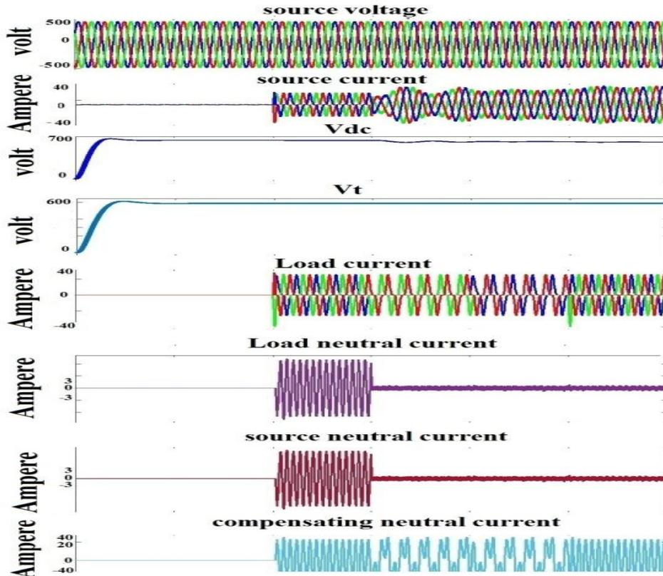
Fig. 4. Output waveforms for balanced Non-linear load.
