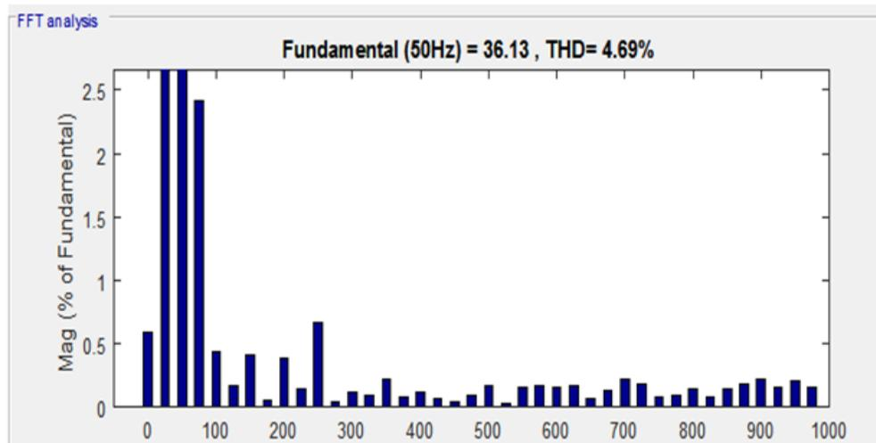
Fig. 7. Frequency analysis of compensated source current for unbalanced load shown 4.69% THD.
