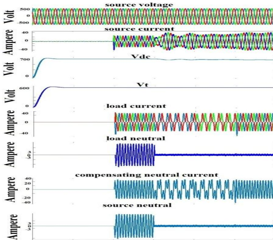
Fig. 6. Output waveforms for unbalanced Non-linear load.
