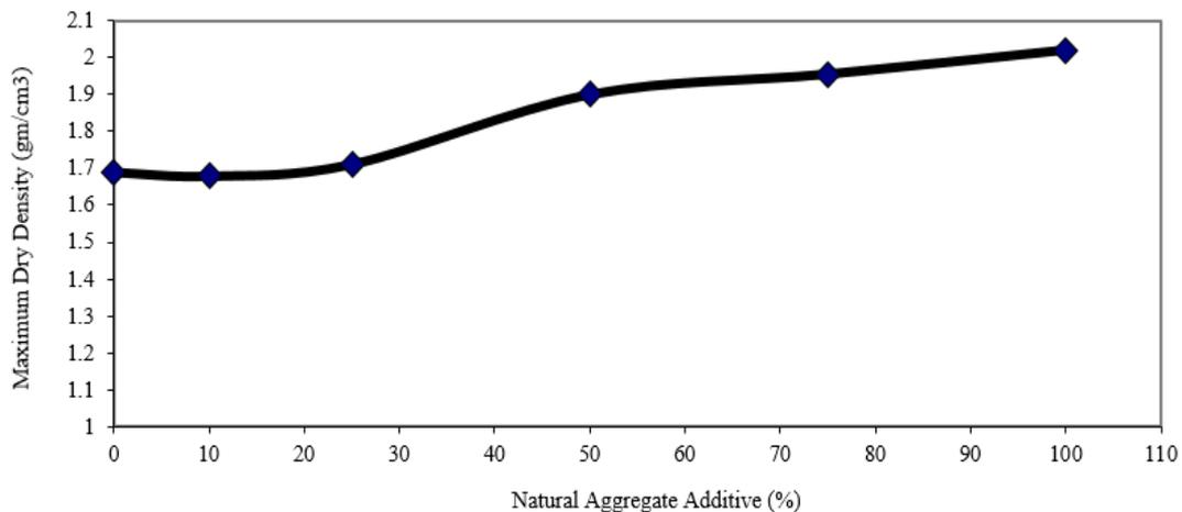
Fig. 6. Relationship between MDD and Add of Proportions of Natural Aggregate to Construction Wastes.
