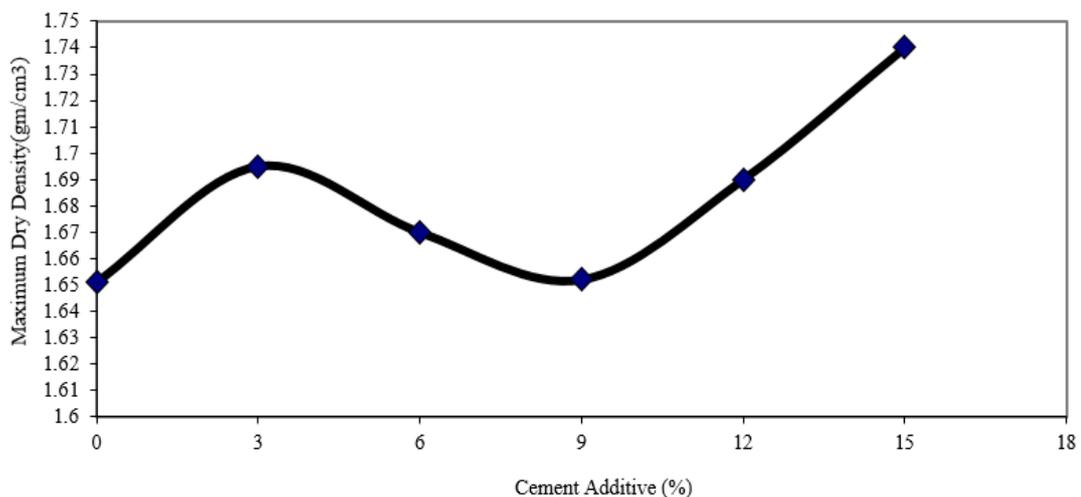
Fig. 8. Relationship between MDD and Add Cement Ratio to Local Soil.
