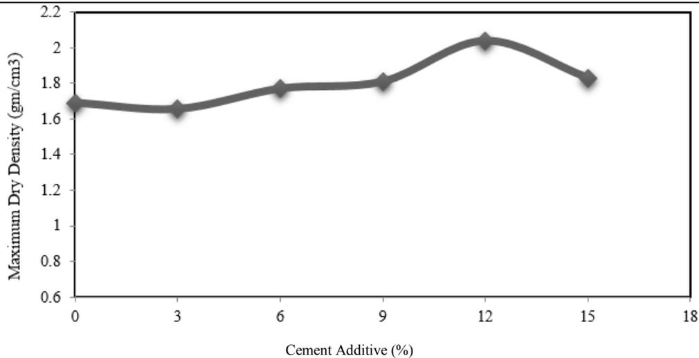
Fig. 2. Relationship Between Cement Additive Add to Construction Wastes and MDD.
