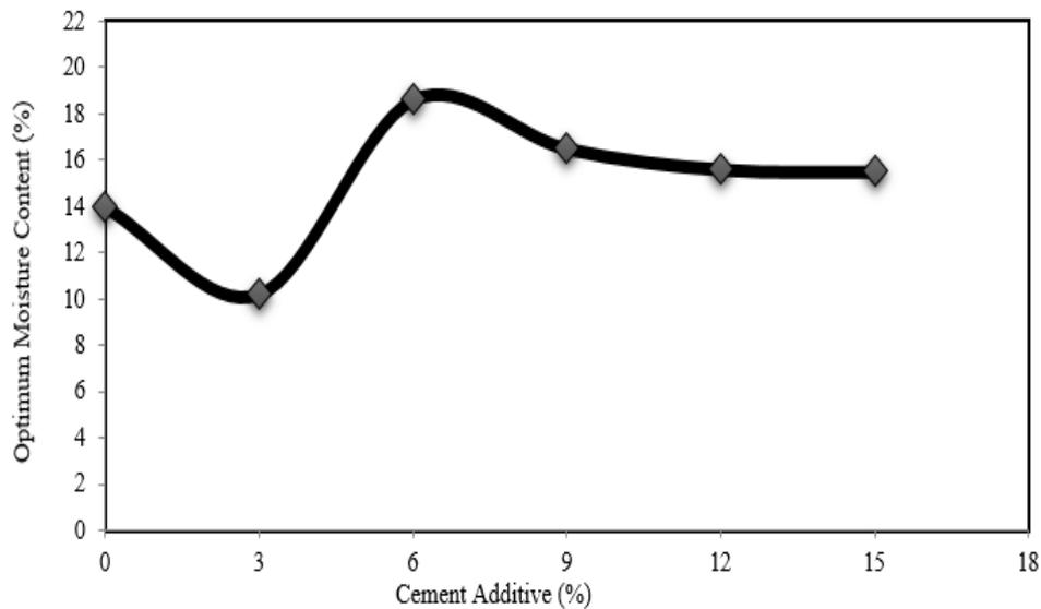
Fig. 3. Relationship between OMC and add of cement proportions to construction wastes.
