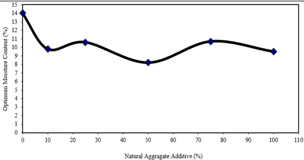
Fig. 7. Relationship between OMC and Add Proportions of Natural Aggregate to Construction wastes.
