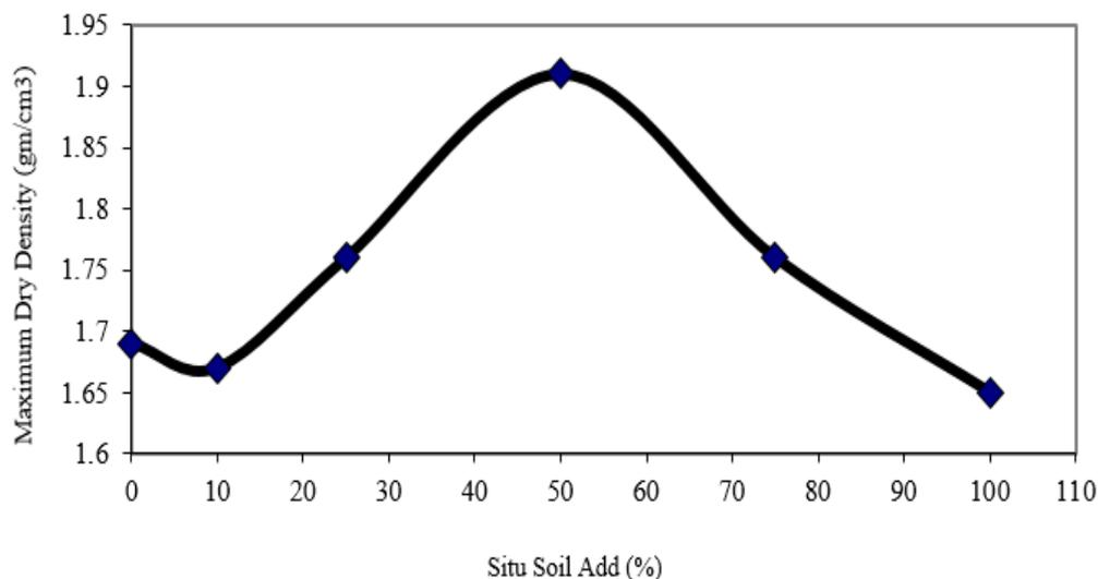
Fig. 4. Relationship between MDD and Add Proportions of Situ Soil to Construction Wastes.
