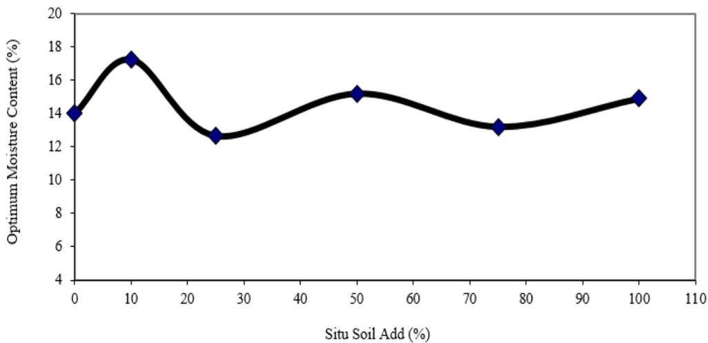
Fig. 5. Relationship between OMC and Add Proportions of Local Soil to Construction Wastes.
