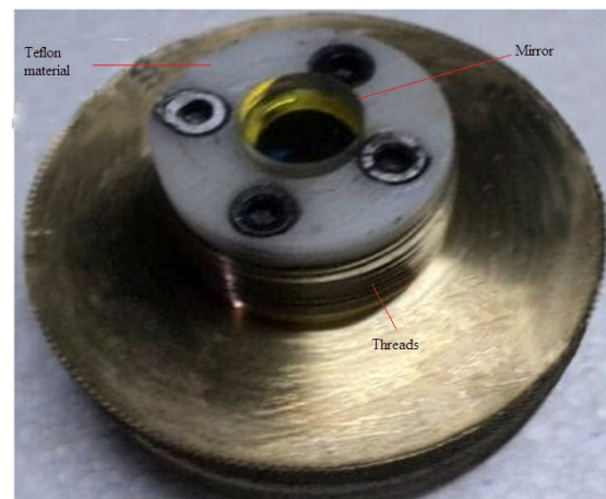
Plate 1: A mirror glued to the adjustable end.
