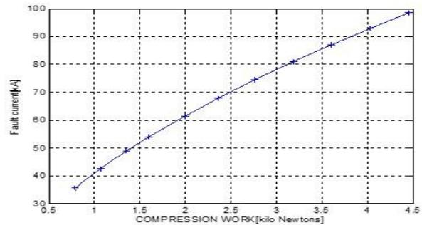
Fig. 4. Response curve of compression work against fault current
