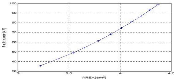
Fig. 3. Response curve of the moving contact area against the fault current
