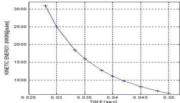
Fig. 1. Response curve of CB total break time ( $t_0$ ) against the kinetic energy requirement ( $W_{KIN}$ )
