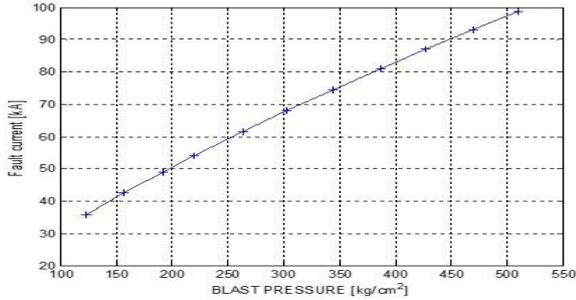
Fig. 2. Response curve of blast pressure against fault current
