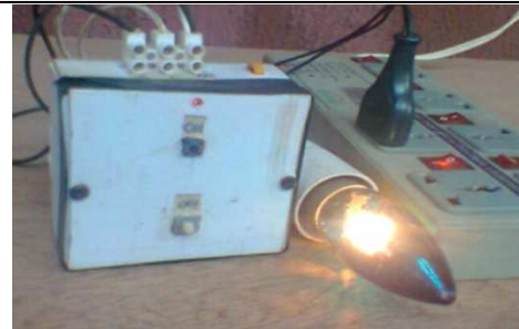
Fig. 3. Test stage 2: Bulb light up, (c) showing present of power when the on button is triggered
