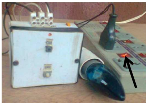
Fig. 2. Test stage 1, power switch is turn on, indicator light on, but no power to the bulb
