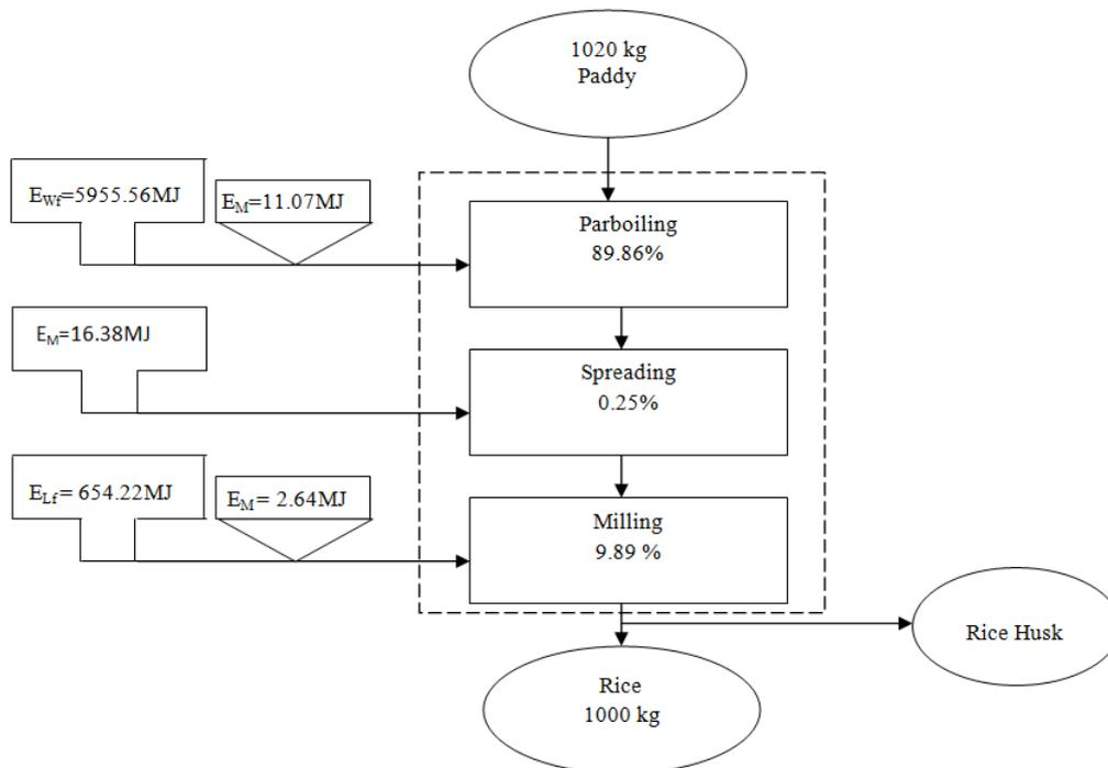
Fig. 2: The Mean Mass/Energy Flow Diagram for the Entire Case Study
