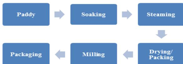
Fig.1. Flow chart showing the unit process for rice milling operation
