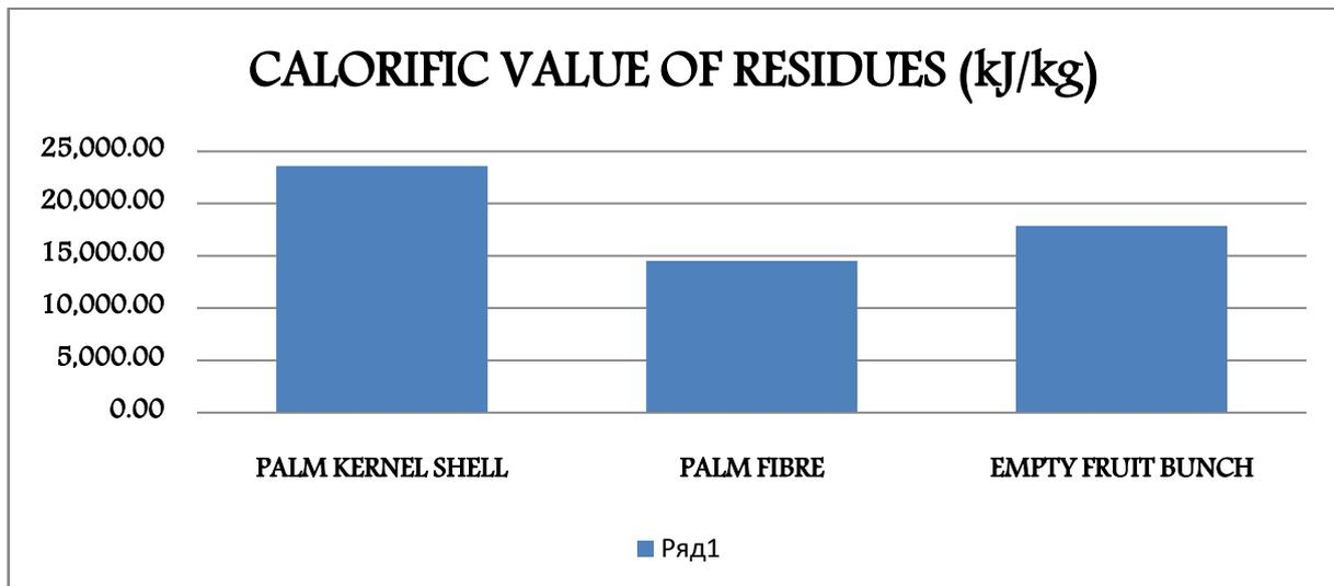
Fig.4. Calorific value of residues
