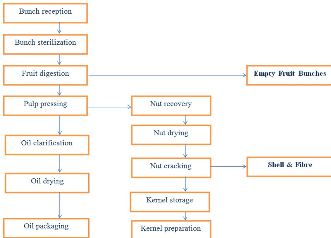
Fig.1. Flow diagram for palm oil processing Source:[11]
