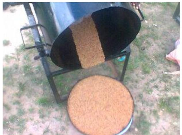
Fig.8. Tilting of steamer to discharge paddy rice
