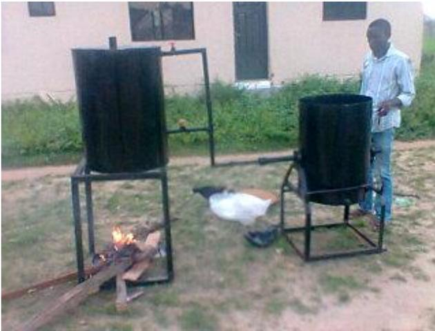
Fig 9: Equipment set-up for parboiling rice
