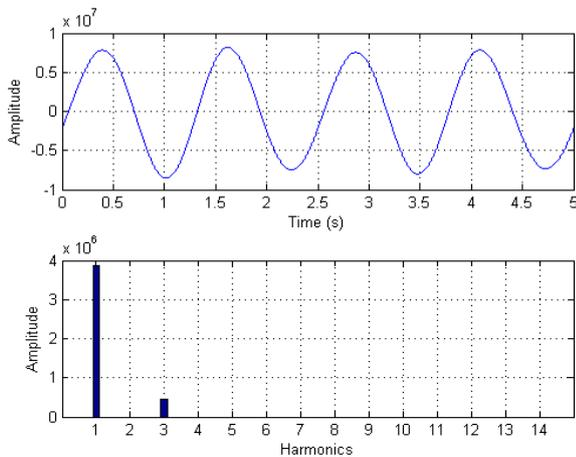
Fig.1.4. (a) Filtered signal after simulation (b) harmonic spectrum filtering
