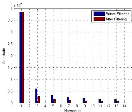
Fig.1.5. Harmonic spectrum before and after filtering
