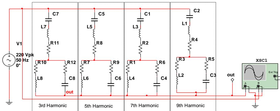
Fig. 1.2 Filter circuit for simulation
