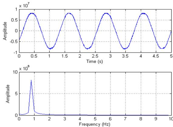
Fig.1.3. (a) Output Voltage Waveform (b) FFT Spectrum of power source
